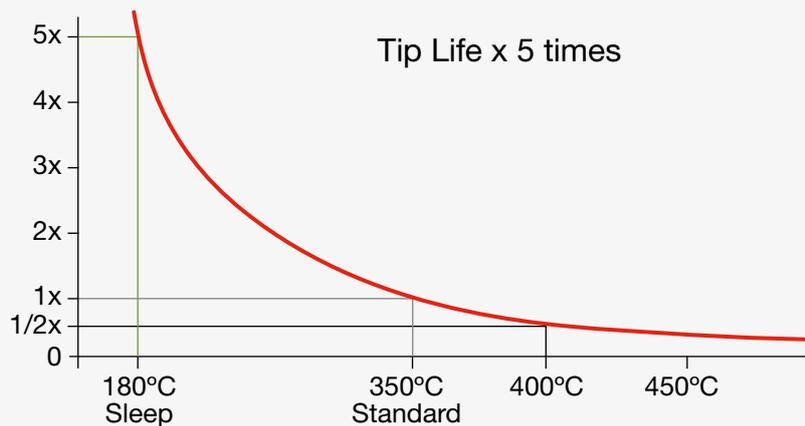
JBC stations features the Sleep & Hibernation functions that lower tip temperature when the tool is not being used. As a result, a tip's life lasts up to 5 times longer. As a result, the tip life increases exponentially.
