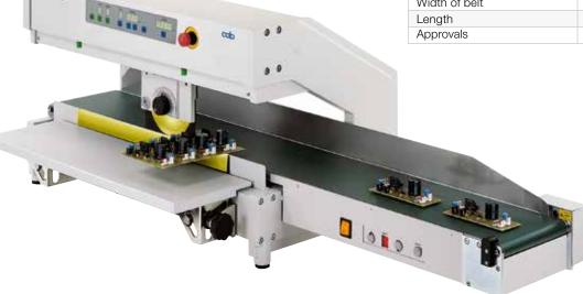
For separating aluminum with the MAESTRO 4S we recommend using the FR4 circular blade with special blade settings. More information in the operation manual and at **www.cab.de/en.**
