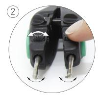
Rotational alignment Turn the cartridges in any direction through the wheels.
