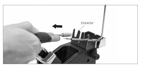
3. Follow the "Placing cartridges" guidelines and use the extractor to help insert the cartridges.
