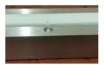
2. Place thermocouple through hole in jaw:
