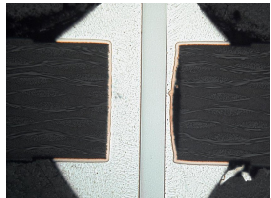
Microsection of CXW-70 lead free alloy, showing a good even fill and even with poor pin placement
