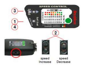
1) Press the Speed button <u>for 2 seconds</u> to visit to PROGRAM mode. Then the two LED lights will display colours depending on the set speed.
