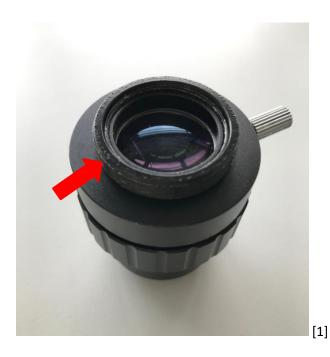
This ring must be detached from the C-mount adapter [2] and put back to the connection point of the camera [3].
