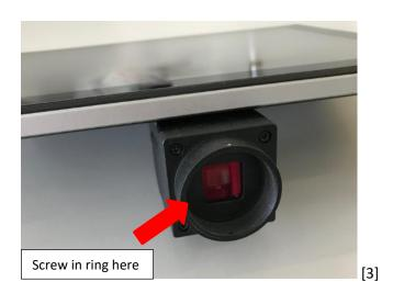
After the ring has been completely screwed back into the circular connection point of the camera, the two Allen screws (0.9 mm) must be tightened [4].
