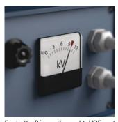
Each Kraftform Kompakt VDE set has been tested individually at 10,000 volts, in accordance with IEC 60900. This ten-times-higher testing load guarantees safe working at their maximum permitted load of 1,000 volts.
