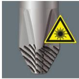
A precisely-focused laser creates a sharp-edged surface structure. This laser treatment results in an edge hardness of up to 1000 HV 0.3. Wera Lasertip "bites" itself into the screw head and prevents any slips out of the recess. It is available for screwdrivers for Phillips and Pozidriv slotted, screws.
