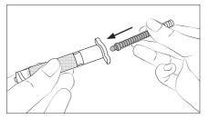
Insert the plunger into te piston and press the piston against the solder paste to eliminate the air inside the barrel.
