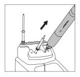
Place the heating element in the extractor and pull the handle to remove it.
