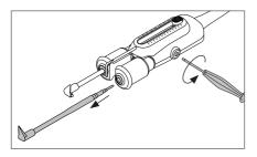
Loosen the screws and remove the cartridges.
