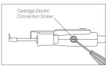
Fix the cartridges in its working position. by tightening the screw.
