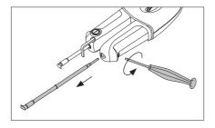
Loosen the screws and remove the cartridges.
