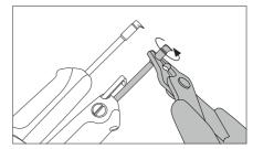
Align cartridges with JBC pliers.
