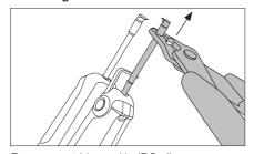
Remove cartridges with JBC pliers.
