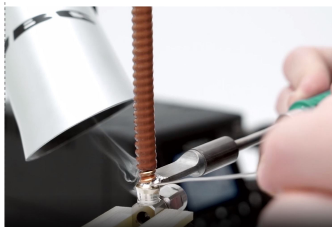
Soldering application using C470012 Cartridge
