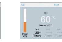
**3** Profile Mode allows control of the heating rate of the PCBA by the use of a control and a protection thermocouple.
