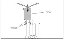
Place the fitters inserted into the grip at the top of the tweezers.
