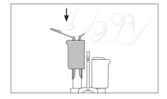
Push the grip with the fitters onto the tweezers.
