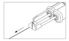
Pull the wire stripper toward to stripp off the wire end.
