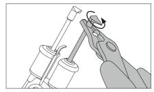
Align cartridges with JBC pliers.
