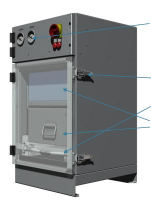
The pressure gauge will indicate the initial (clean) pressure of the system.
