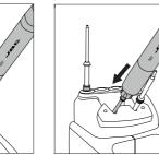
Place the handpiece on top of the new heating element and press down slightly.
