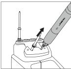
Place the heating element in the extractor and pull the handle to remove it. 2. Inserting
