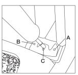
Use the holes for fixing the cartridge<sup>\*</sup> as follows: **A.** For straight C210. **B.** For curved C210. **C.** For C245.
