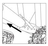
Place the handpiece in the extractor and pull to remove the cartridge.
