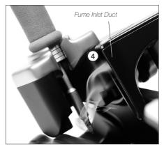
4 The system detects when the tool is returned to the station and the fume inlet duct automatically absorbs the fumes.
