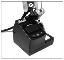
2 Insert the fume inlet duct for compact stations between the knob and the tool holder.
