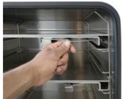
Figure 10: Operating the expansion racks
