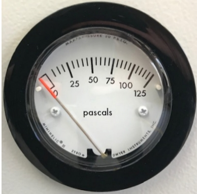
Figure 23: Analog pressure display (manometer) for monitoring the compressed air flushing on the chamber front
