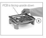
Then tilt the holder all the way back (3) until it comes to rest in a horizontal position again (4).
