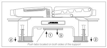
Lift the support while holding the tabs and let its feets drop down under their own weight (2).
