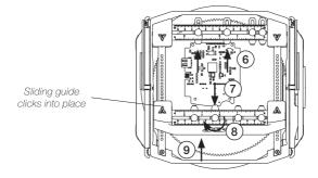
Now adjust the positions of the other requiered slot clamps to the PCB shape and tighten their clamp knobs (10) after the adjustment.
