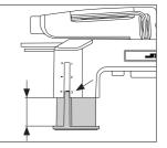
To adjust the height, press the two lower push tabs upward at the same time and hold them pressed (1).
