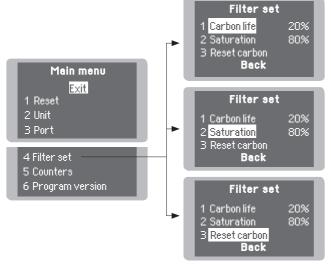
Shows % of remaining life of the carbon filter contained inside the FAE1-200 filter. It is also displayed on the main screen.
