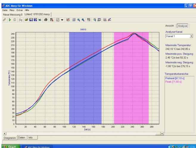
Temperature profile with coloured marked temperature areas
