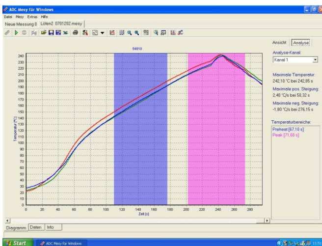
Temperature profile with coloured marked temperature areas
