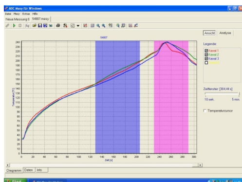
Typical lead free profile 548.07G
